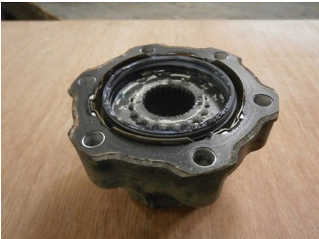
Un-locked hub with centre gear in 2WD position (held in position with magnet built into hub)
