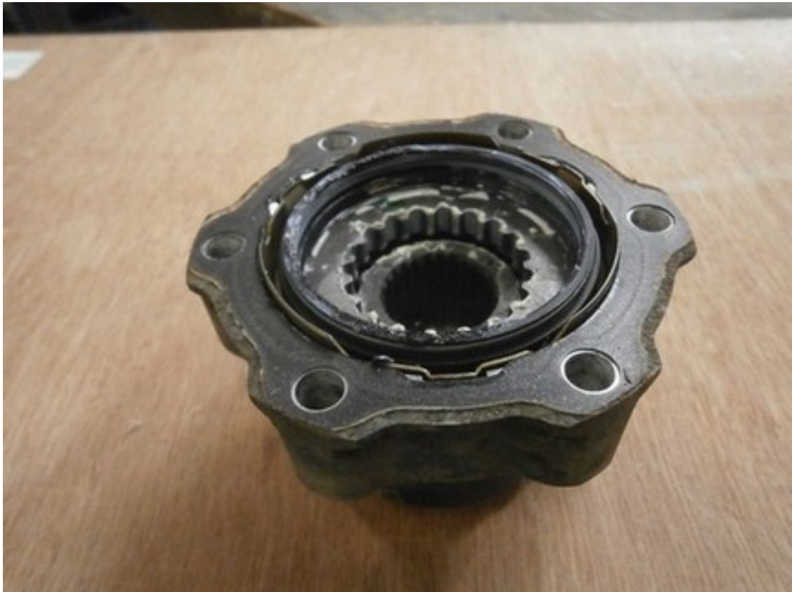
Un-locked hub with centre gear in 2WD position (held in position with magnet built into hub)
