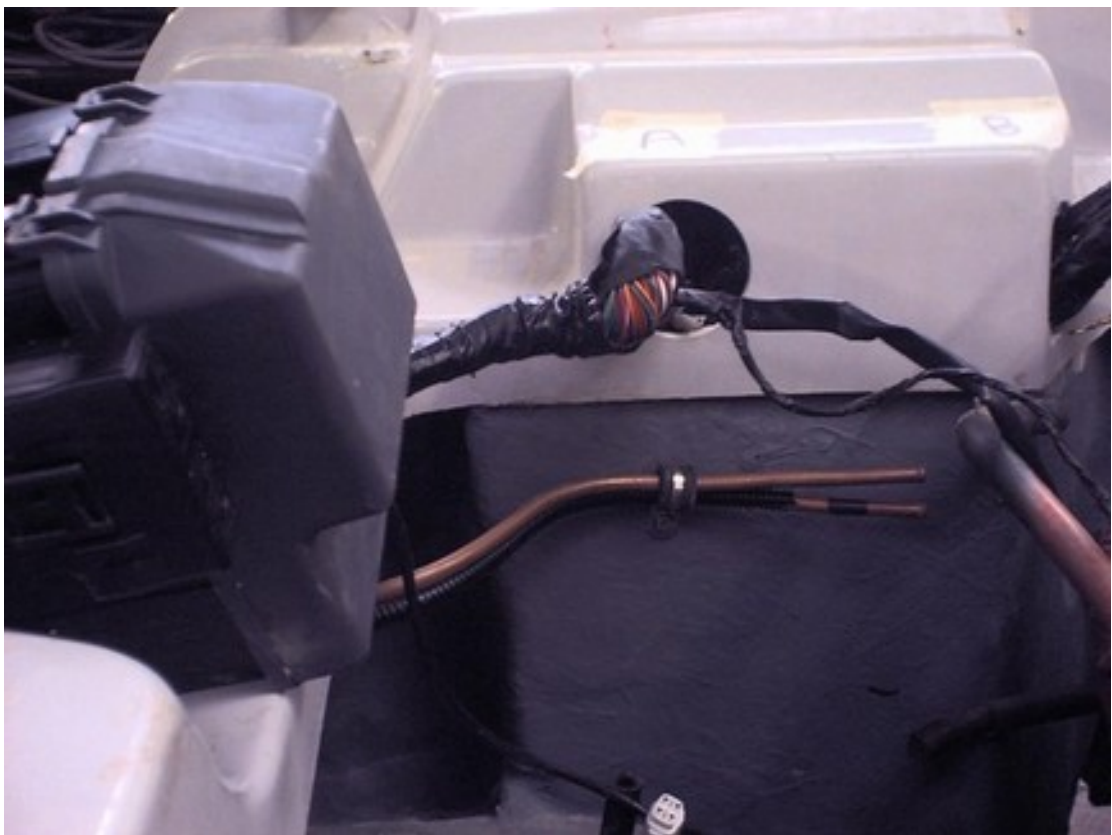
Bolt up controller box and immobiliser box
