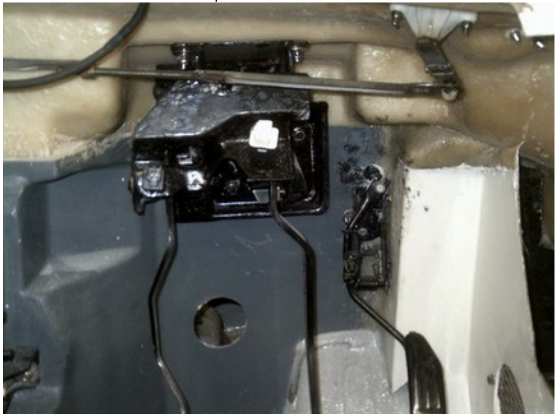
LEFT HAND DRIVE bend accel pedal to clear GRP
