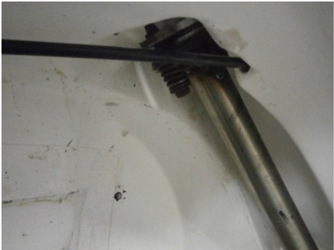
cross cable is steering Morse to rudder factory fitted
