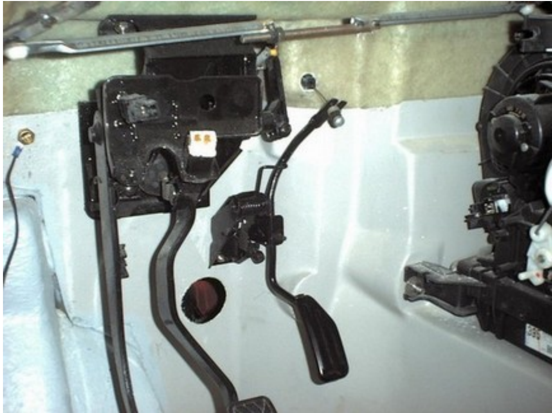
LEFT HAND DRIVE bend accel pedal to clear GRP
