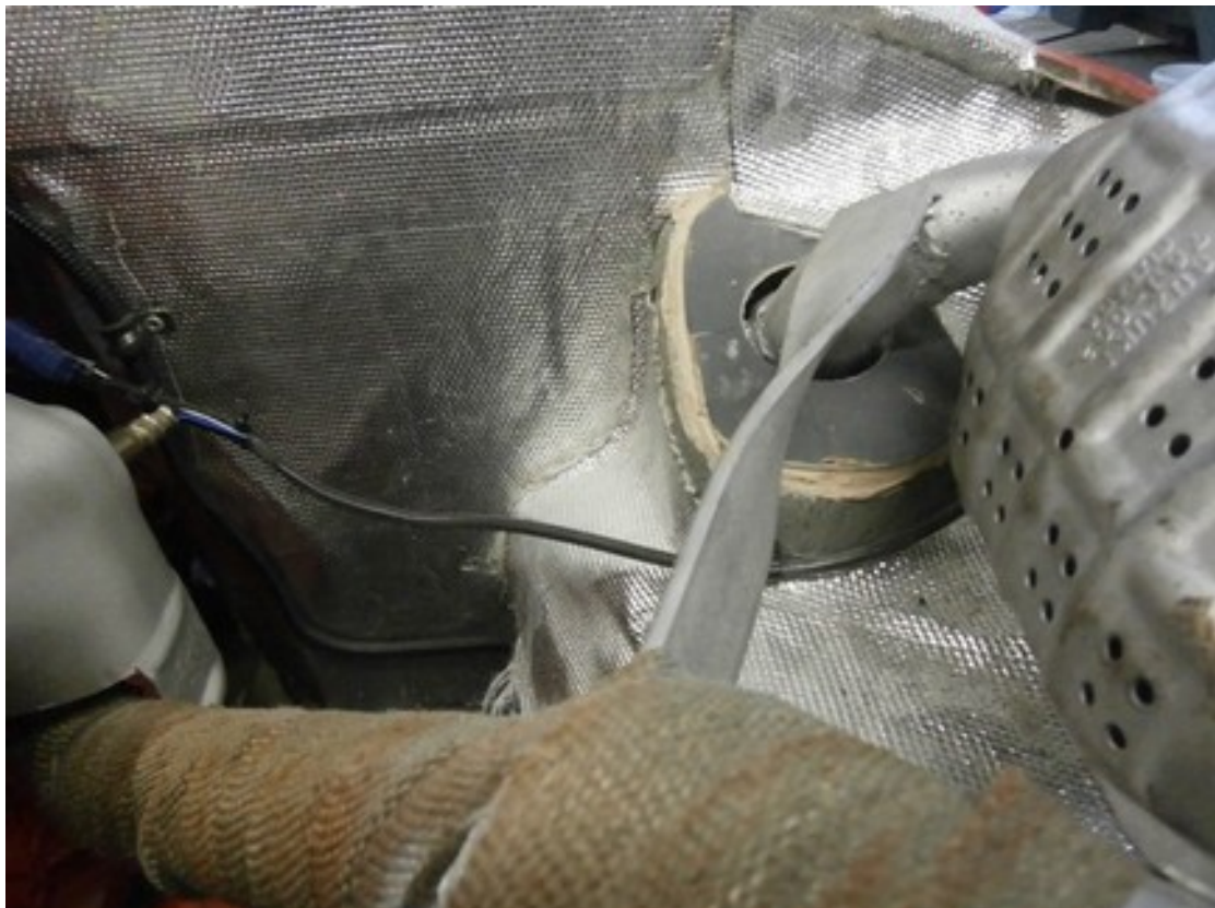
Mastic or body filler GRP panel to hull leave 1/4" gap around pipe for engine movement
