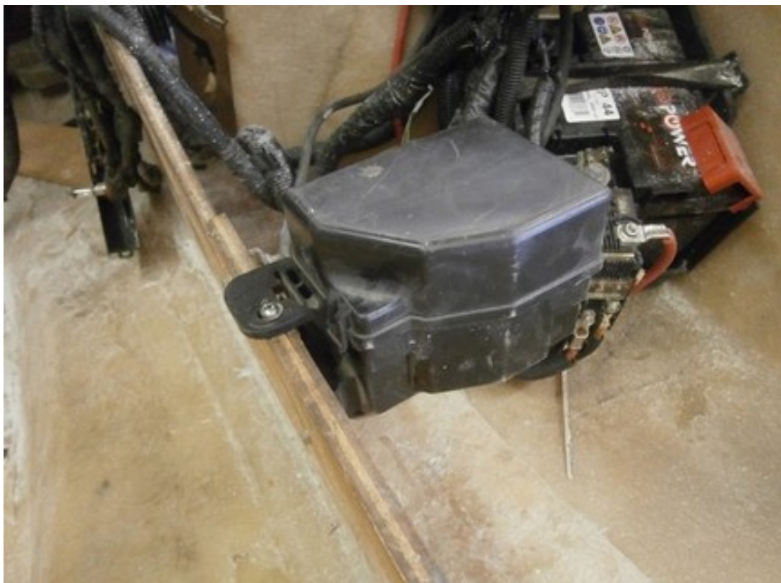
Fit 2 nd fuse box on side of timber. Not fitted to all Fiestas
