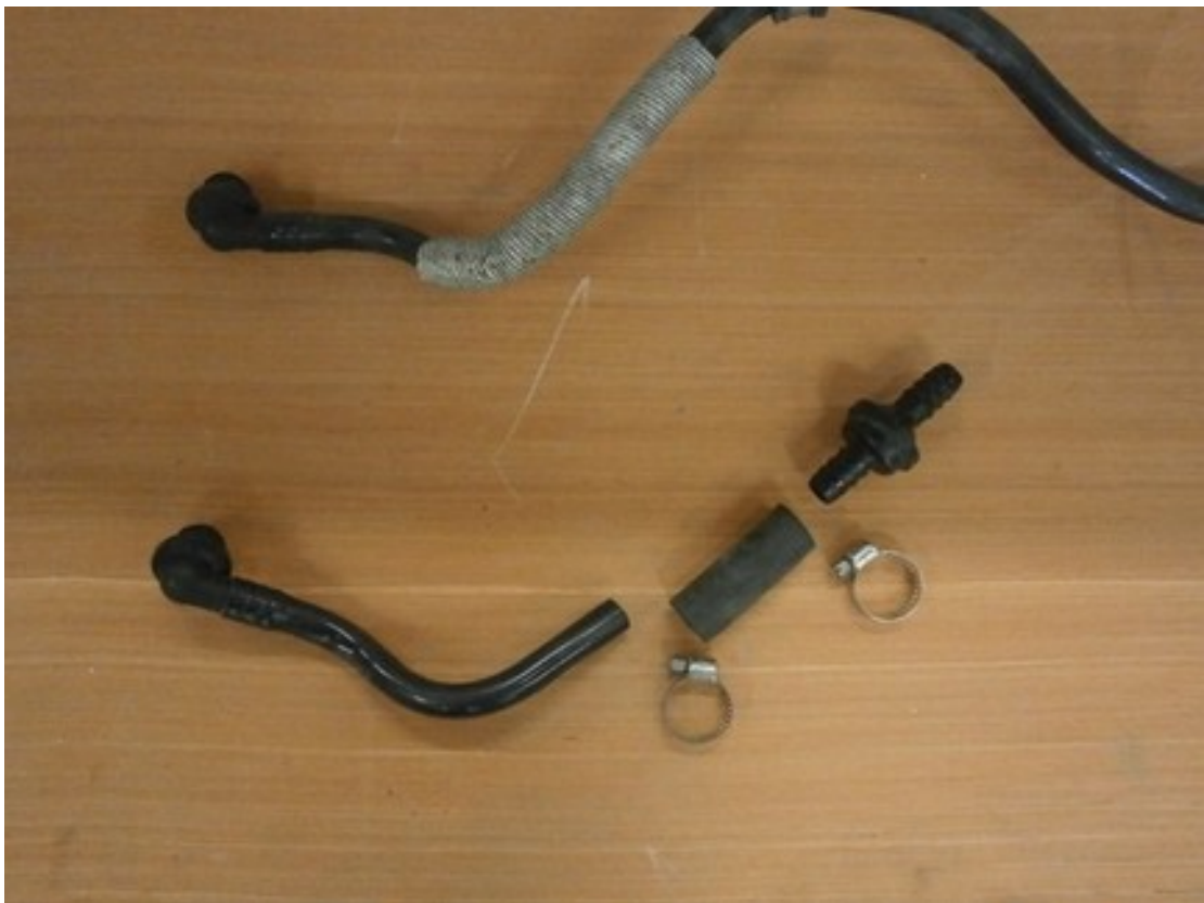
Cut servo end of plastic hose. Fit one way valve using 2" rubber hose and clips. Check major diameter is towards engine
