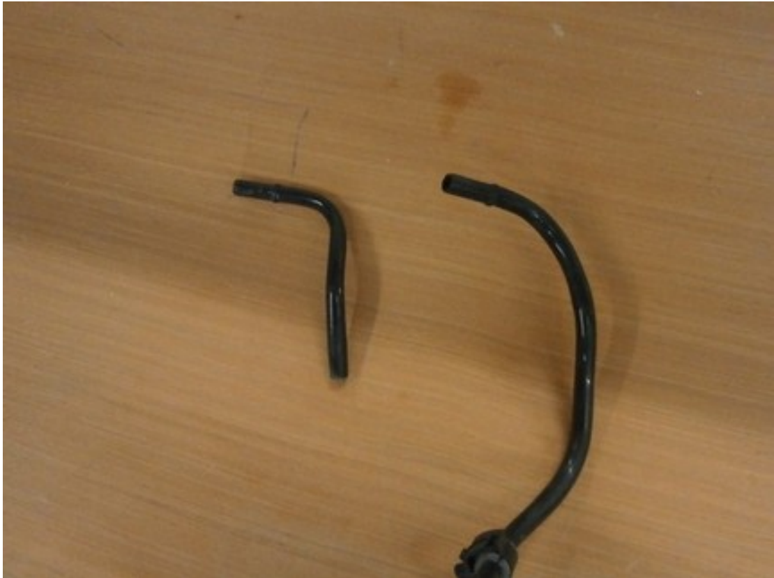
Cut engine end of plastic hose
