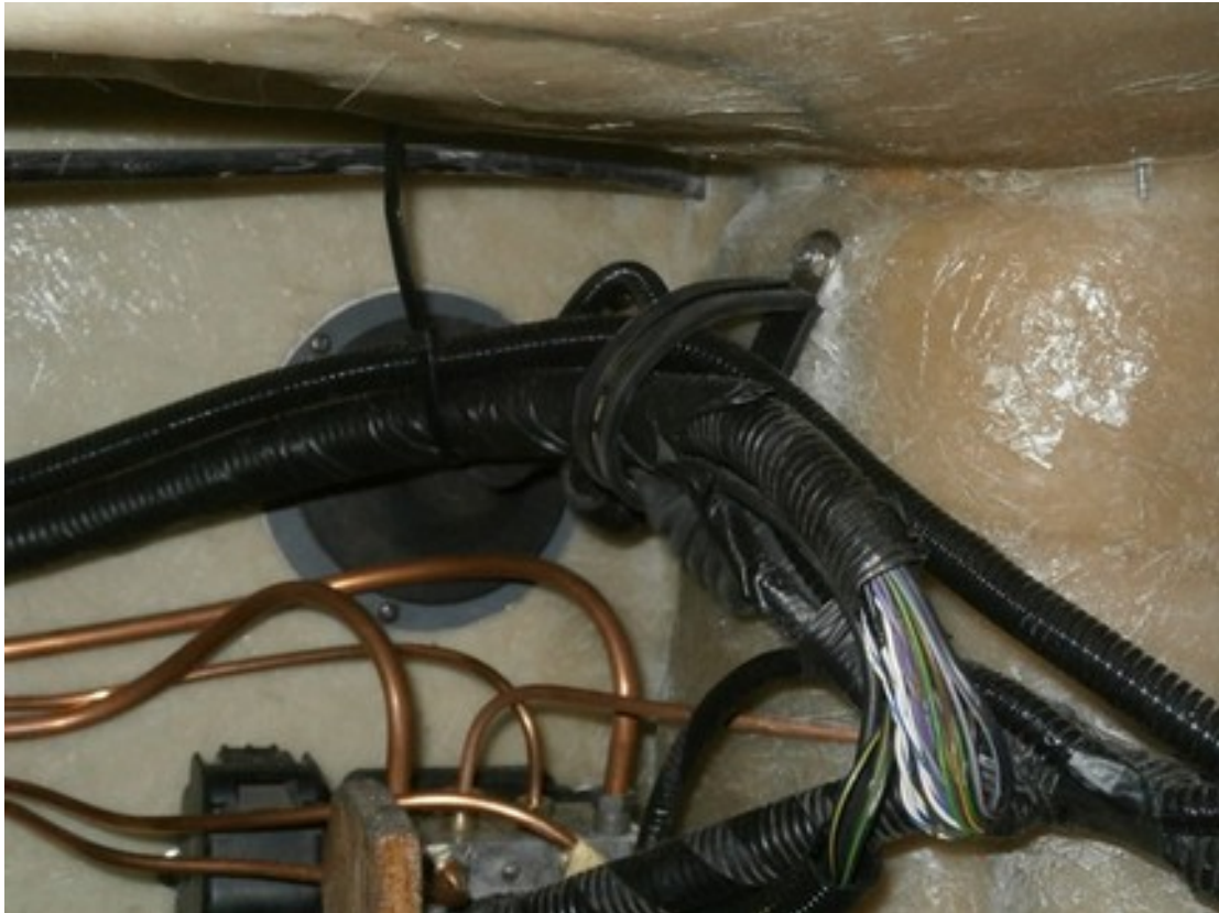
Fit 2" P clip as shown to clear brake pipes and tank GRP
