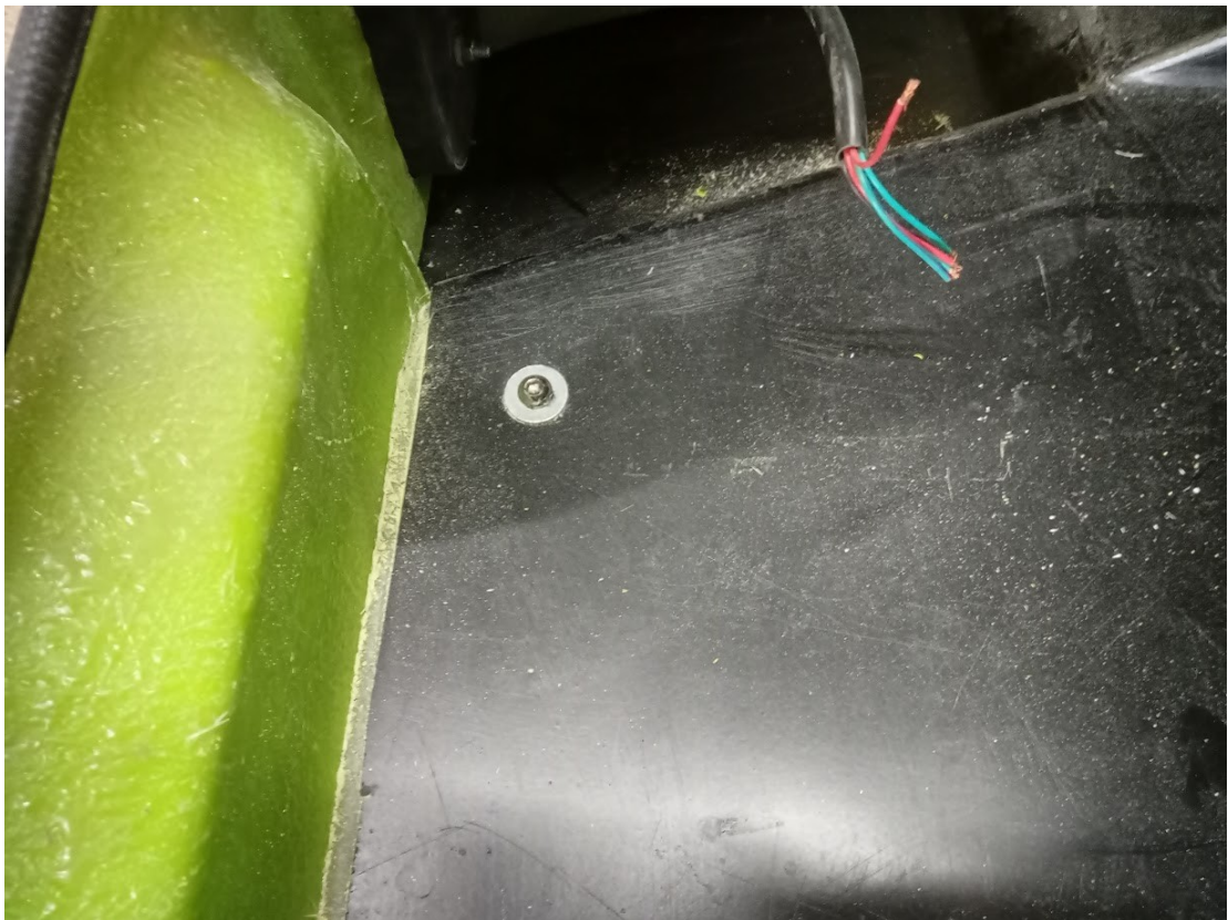
Re-bolt body to chassis
