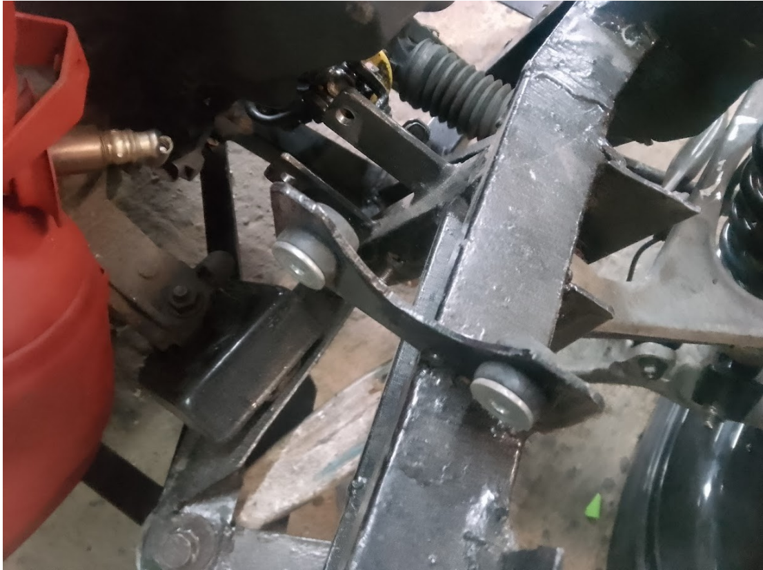
Fit Mazda rubber insulators and sleeves into bracket on chassis
