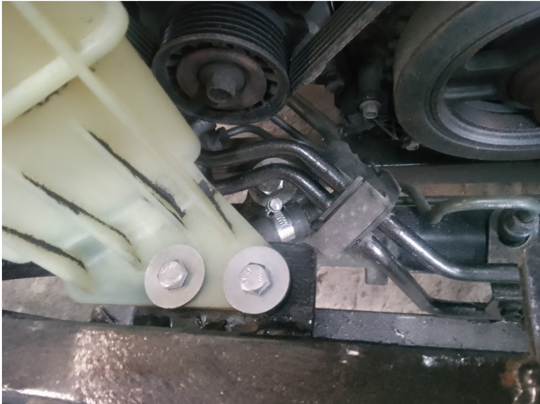
bolt power steering bottle 2 off M6 x 25 and couple up hydraulic hoses. Discard separate steel oil heat exchanger tube
