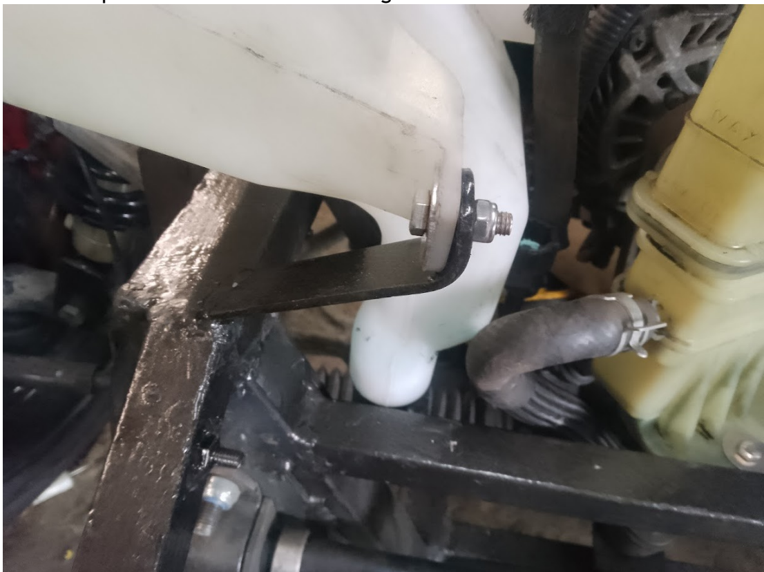
bolt power steering bottle 2 off M6 x 25 and couple up hydraulic hoses. Discard separate steel oil heat exchanger tube
