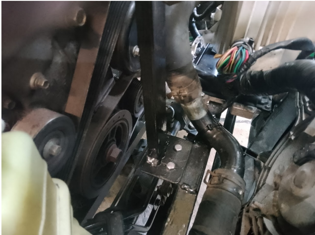
bolt steel water tank bracket to chassis 2 x M6 x 25
