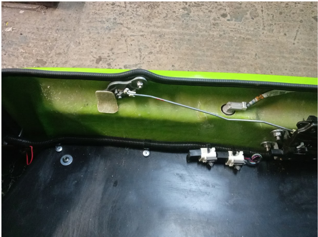
bolt manual key operate lock to pre-drilled holes. Bolt striker plate to boot lid. Adjust to suit
